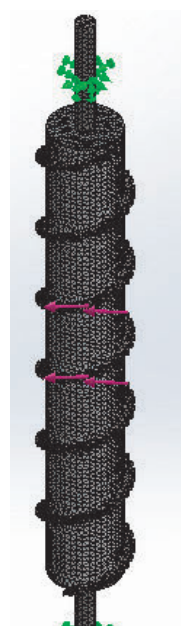
Fig. 3. Mesh model, fixed member (by green narrows) and applied torque (indicated by pink arrows) in dehiscing roll
